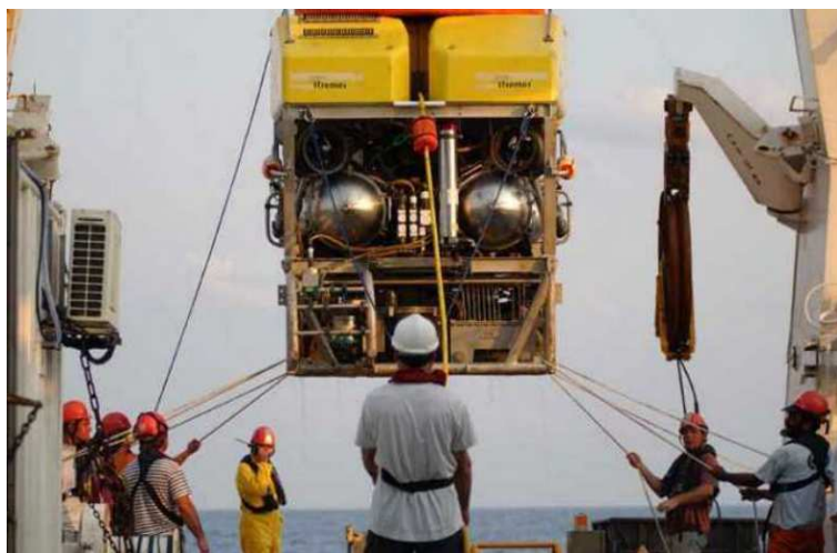
Figure 2. The deep-sea ROV, VICTOR 6000
